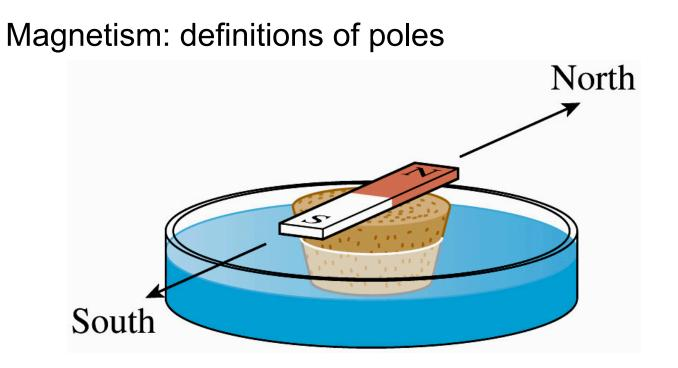
Put bar magnet on a cork and float it in a dish of water.
