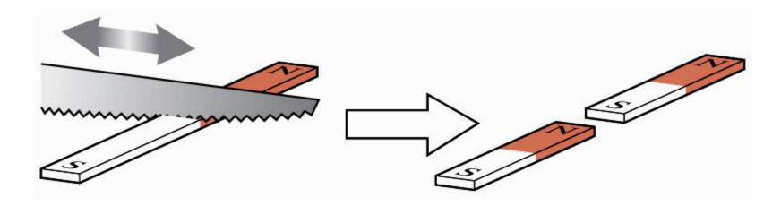
Cut a bar magnet in half. Can you isolate the north pole and the south pole on separate pieces?
