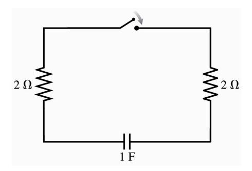
The 1F capacitor is initially charged with 2 C. The time constant for the discharge of this capacitor is:
