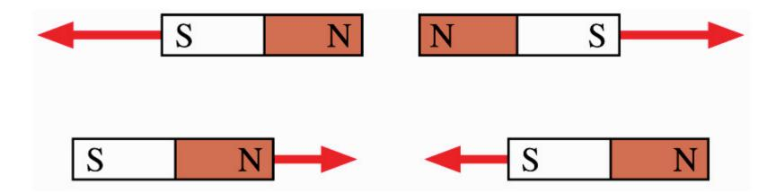
Bring the north poles of two bar magnets near to each other. Then bring the north pole of one magnet near the south pole of another magnet.
