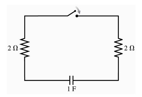
The 1F capacitor is initially charged with 1 C. The time constant for the discharge of this capacitor is:
