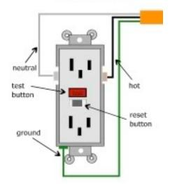
Wiring conventions: Black wire = "hot" White = "neutral" (*should* be grounded) Green = ground (*must* be grounded)
