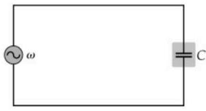
2) Figure above shows a simple ac circuit composed of a capacitor connected across the terminals of an ac generator. If the frequency (in Hz) of the generator is doubled, what happens to the capacitive reactance of the capacitor?
