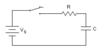
13) (8 pts) A 4.0  $\mu$ F capacitor C is connected in series with a 2.0 k $\Omega$  resistor R, across a 20-V DC source and an open switch, as shown above.
