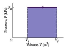
6. (6 pts) A monatomic ideal gas expands from an initial volume of 30.0 L to a final volume of 65.0 L, at a constant pressure of 110 kPa. How much work is done by the gas?
