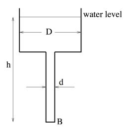
For 3-4: Two containers have a shape like that shown above. Both are filled up to the level marked *h*, and have identical narrow tubes with diameter *d*. However, they have **different** values of the diameter of the upper cups, *D*. The pressure at the bottom of the tube at point B is measured in both containers.
