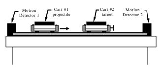
velocity of Cart #1 is 40.0 cm/s and the velocity of Cart #2 is 0.00 cm/s. The carts collide and Velcro surfaces of the carts stick together, so that the pair of connected carts continues to move to the right on the track.
