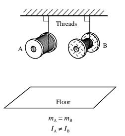
The linear acceleration is related to the angular acceleration by a factor of the radius out to which the thread is wrapped. (i.e.  $a = \alpha r$ ) For B to have a larger linear acceleration with a smaller radius, it must have a larger angular acceleration.
