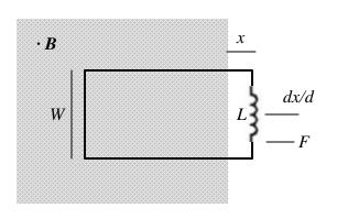
15. [20] Show that the force required to pull the loop is given by  $F = W^2 B^2 x/L$ .
