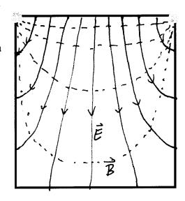
6. [10] At a frequency low enough that only this one mode can propagate, sketch on the diagram the electric and magnetic field lines inside at some instant in time. Remember to take into account the boundary conditions on E and B. Also, what can you say about the field components along the tube?
