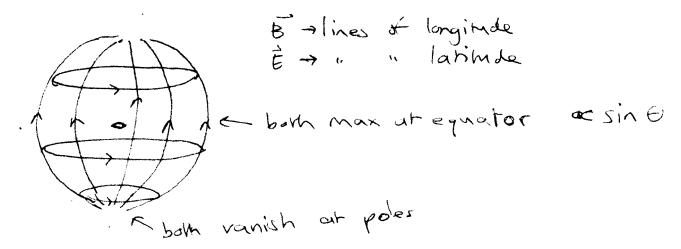
The instantaneous Poynting vector at point  $(\mathbf{r},t)$  for a source of size *L* located at the origin is given approximately by the following, where  $\mathbf{p}(t_r)$  is the dipole moment of the source at the retarded time:
