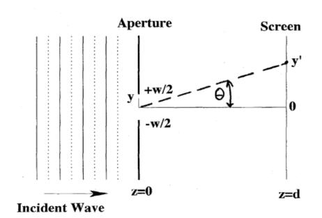
Plane wave diffraction. Wavelength, 1  $\mu$ m. Slit width, 10  $\mu$ m. Source to detector plane separation: 1 m.
