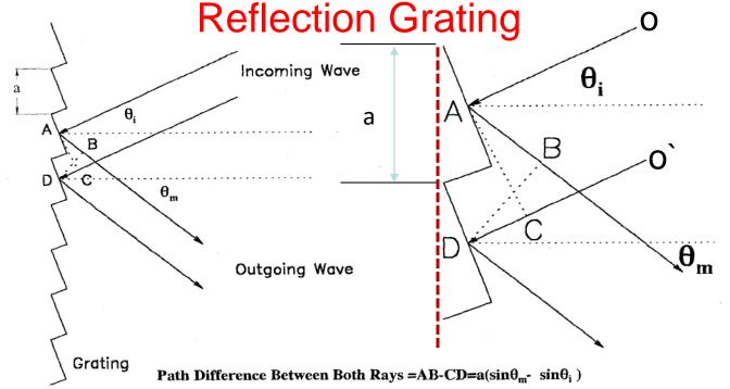
Grating spacing = a, incoming angle =  $\theta_i$ , outgoing angle =  $\theta_m$ Constructive Interference from two facets occurs when:
