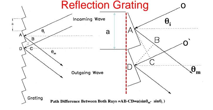
Electric Field from N facets: (Define:  $\alpha \equiv$  one half phase difference between successive waves= $\frac{ka}{2}(\sin\theta_m - \sin\theta_i)$
