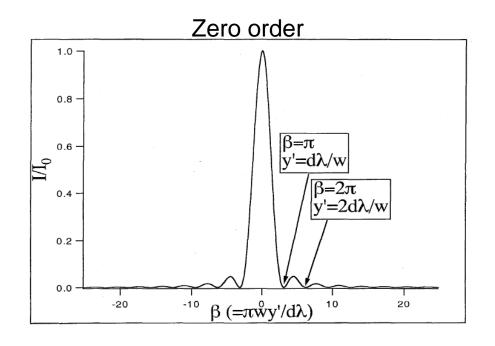
Important concept: most energy is stored in zero order, which is useless for distinguishing different wavelengths.
