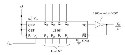
As before, look up the datasheet for the LS161 and determine its pinout and use it to wire up the circuit above. Use a debounced switch or the SYNC OUT of the function generator for  $f_{in}$  Use the HP display or the 4-LED array (your choice). For the inverter, use a 74LS00 wired appropriately.
