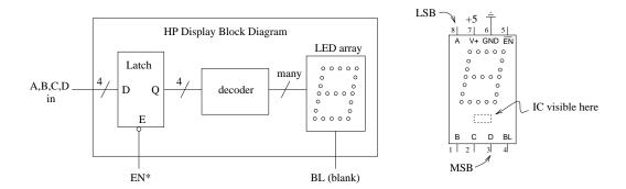
The display chip is more than just a seven segment LED, It has a decoder that translates the binary number input to A, B, C and D into the proper pattern, and it includes a transparent latch that allows the number to be loaded on the assertion of EN\* and saved when EN\* is disasserted (note "assert" means "set to LOW"). There is also a blank pin that when asserted will cause the LEDs to turn off. You can see the IC in the face of the chip that tells you which side is down.
