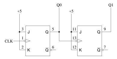
Check that  $\overline{S}$  and  $\overline{R}$  are disasserted for both flops (they should be, already).
