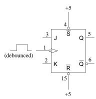
Be sure to wire the  $\overline{S}$  and  $\overline{R}$  inputs of both flops in the package to high. See the pinout diagram on the laminated sheets in the lab ("CLR" is the same as  $\overline{R}$ ).
