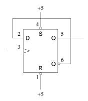
Remove the manual clock connection and clock the flop with the TTL output of the function generator (SYNC). Watch both the clock and Q lines on the 'scope and draw the two waveforms you see. Why is this circuit called a "divide-by-two"?
