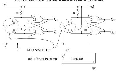
After wiring up the debounced switches, confirm that the outputs go cleanly between HIGH and LOW as you flip the toggle switches. (You can confirm that the input switches actually
