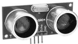
A complete data sheet is included with this write up at the end. Briefly, to use the device, a measurement is initiated by a positive going pulse on the trigger line. A short time later, the Echo line goes high and gives a pulse proportional to the distance between the sonic ranger and the nearest echo-able object.
