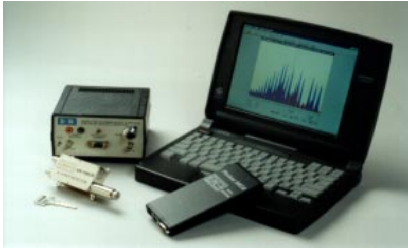
Figure 12. XR100CR, MCA8000A, and Laptop Computer
