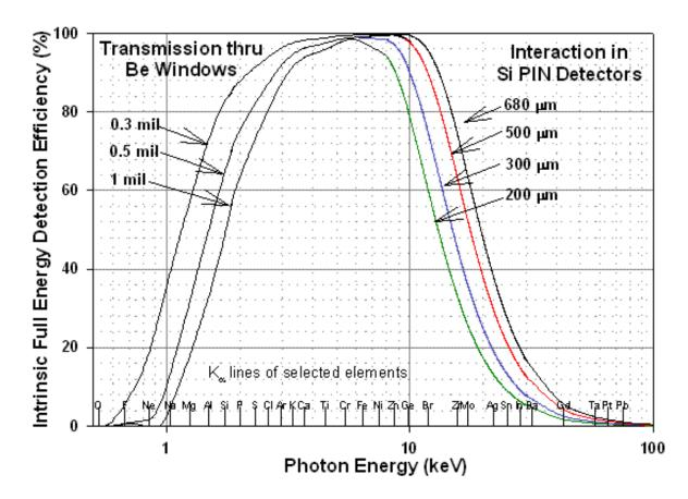
This shows the intrinsic full energy detection efficiency for the XR-100CR detectors. This efficiency corresponds to the probability that an X-ray will enter the front of the detector and deposit all of its energy inside the detector via the photoelectric effect.
