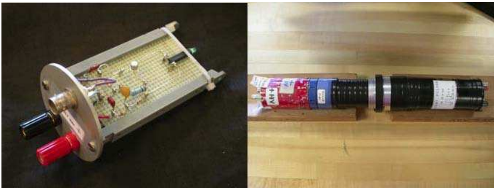
Figure 1: Left: Light pulser module. Note the little LED at the end opposite the terminals. Right: PMT inserted into the light-pulsar housing (not taped up, though).
