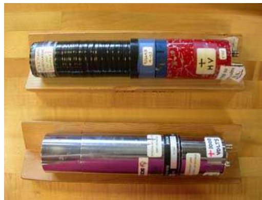
Figure 2: Top: Plastic scintillator detector. Bottom: Bicorn NaI detector.
