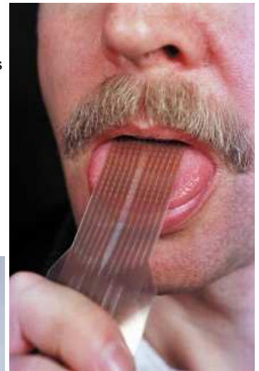
At the end of a flexible cable pressed against the tongue, an array of dotlike metal electrodes (below) stimulates touch-sensitive nerves with electric pulses. Patterns of pulses represent images from a video camera (not shown). J. Miller
