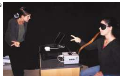
Blindfolded but tongue-tuned to a video camera (white box beside laptop), Alyssa Koehler mimics hand gestures by Sara Lindaas. These sighted, occupational-therapy students are part of a team devising a curriculum to train blind children to use the image-translating system. K. Kamm/U. Wis.-Milwaukee
