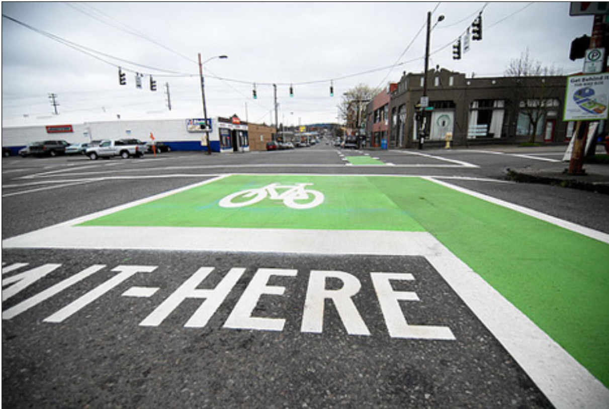
Figure T-14. Advanced stop line or “bike box” in Portland. Source: BikePortland.org.
