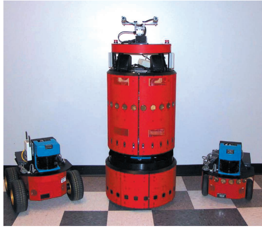
Figure 4. Robots have many onboard sensors for use in localization, multirobot collaboration, and zero-knowledge map building.
