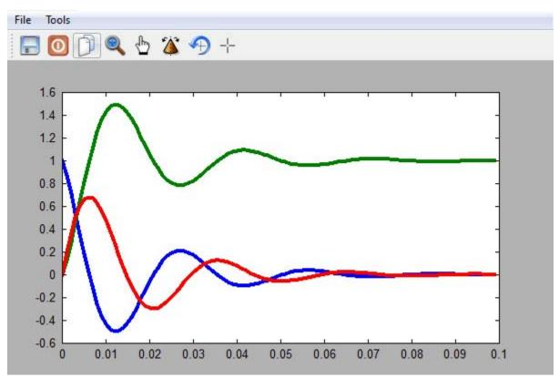
Blue is natural, green is step, and red is impulse response. The vertical axis is in millimeters.
