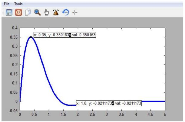
The plot that we have here is equivalent to a unit impulse response of a standard second order system, such as a series RLC circuit. However, because of the derivative term in the controller, there is an extra "s" factor in the numerator. When the input is a unit step, the LT of that step (1/s) cancels out the "s" so there is no 1/s term after we do partial fractions.
