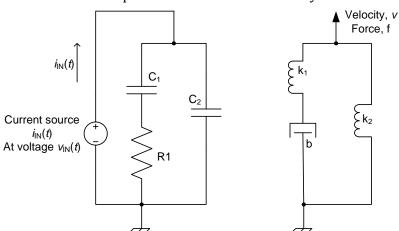
Schematic drawings of electric circuit (left) and mechanical system (right). Spring constants are represented by *k* and the ratio of force to velocity is *b*.
