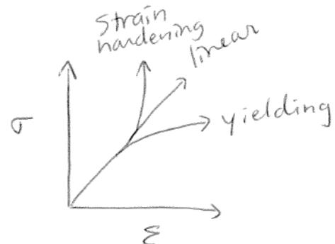
The fractional change in length after stress is removed is called **residual strain**. Irreversible deformation like this is referred to as **plastic deformation**.
