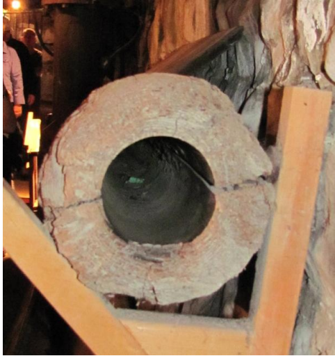
Figure 2: A cross-section image of a wooden pipe.
