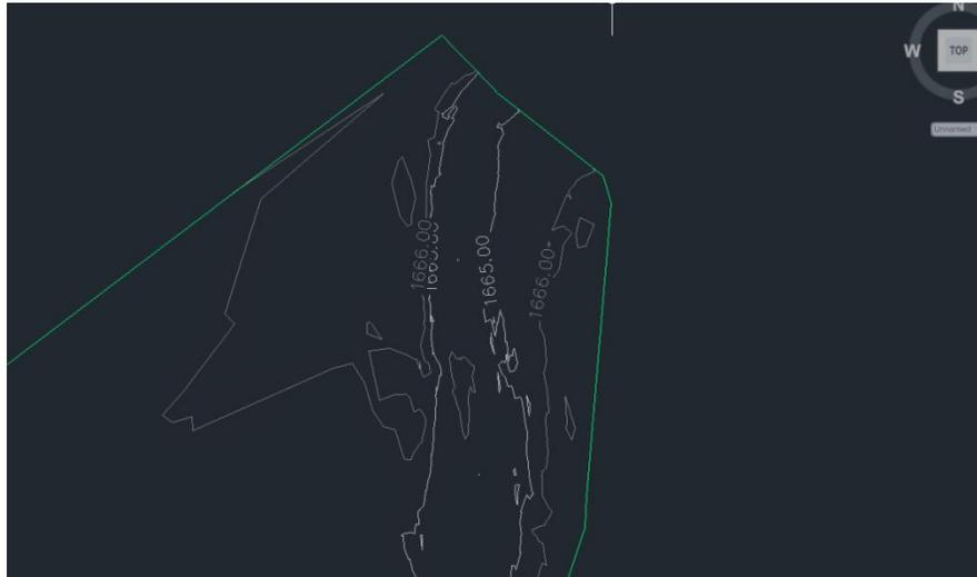
As expected, the slope is draining to the river from both sides (1666 m to 1665 m).
