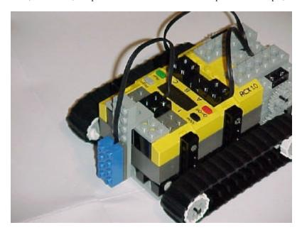
We also need the race track that comes with the RIS kit (This big piece of paper with the black track on it.) The idea now is that the robot makes sure that the light sensor stays above the track. Whenever the intensity of the light goes up, the light sensor is off the track and we need to adapt the direction. Here is a very simple program for this that only works if we travel around the track in clockwise direction.
