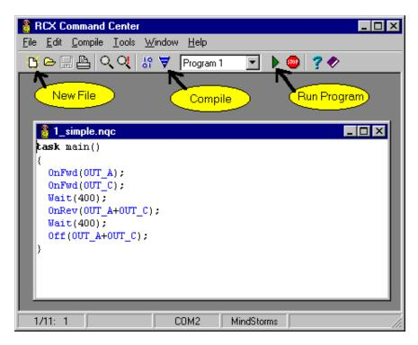
The interface looks like a standard text editor, with the usual menu's, and buttons to open and save files, print files, edit files, etc. But there are also some special menus for compiling and downloading programs to the robot and for getting information from the robot. You can ignore these for the moment.
