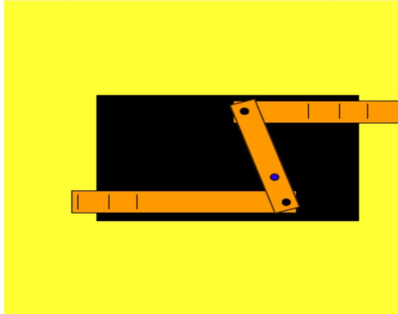
When lever "A" is pushed in 2 cms Lever "B" moves in 1cm.
