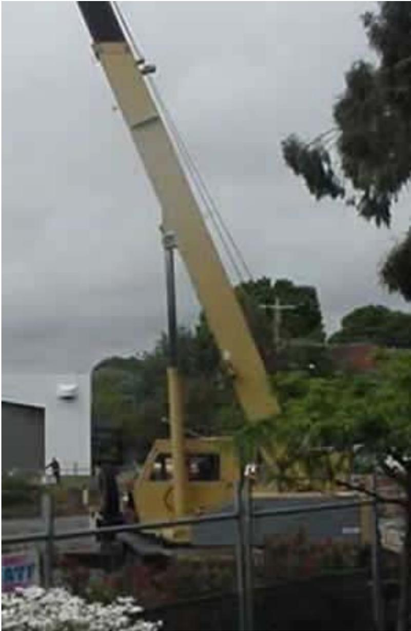
Cranes such as the one on the left are examples of third order levers. As you can see the effort is between the load, at the top, and the fulcrum. The advantage of this lever system is that the load moves through a greater distance than the effort. This is desirable when the crane needs to lift loads high above the ground.
