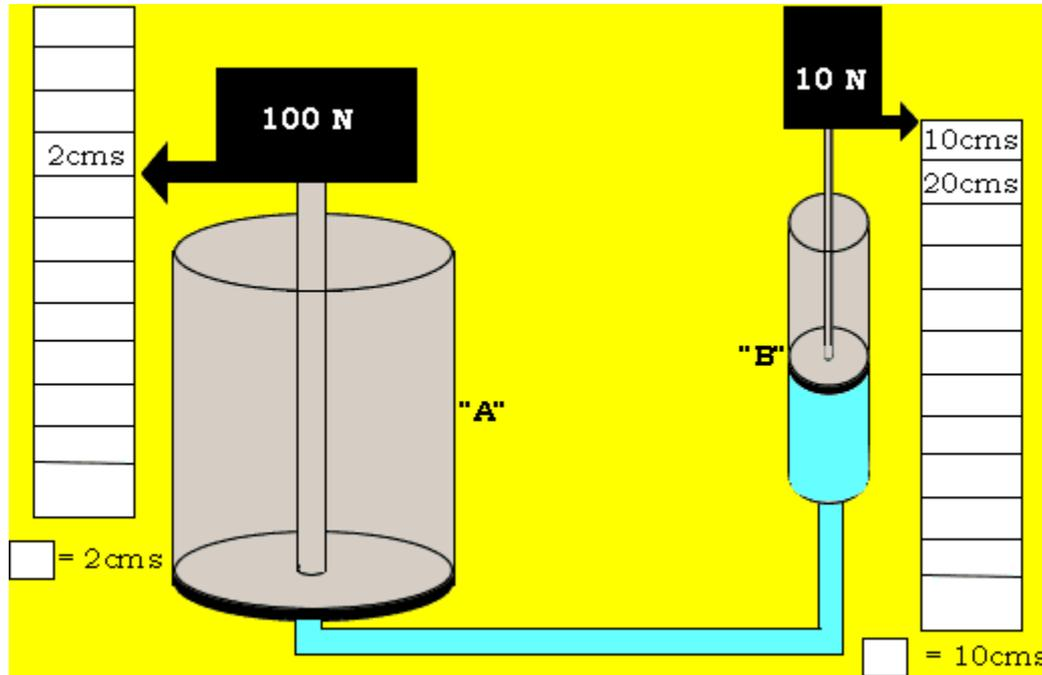
Look at the operation of the two pistons above of a 10N force being multiplied to become a 100N force. Notice how the smaller piston with a force 10N travels 20cms down the grid, while the larger pistons travels 2cms up the grid. Now lets calculate the work done by each piston.
