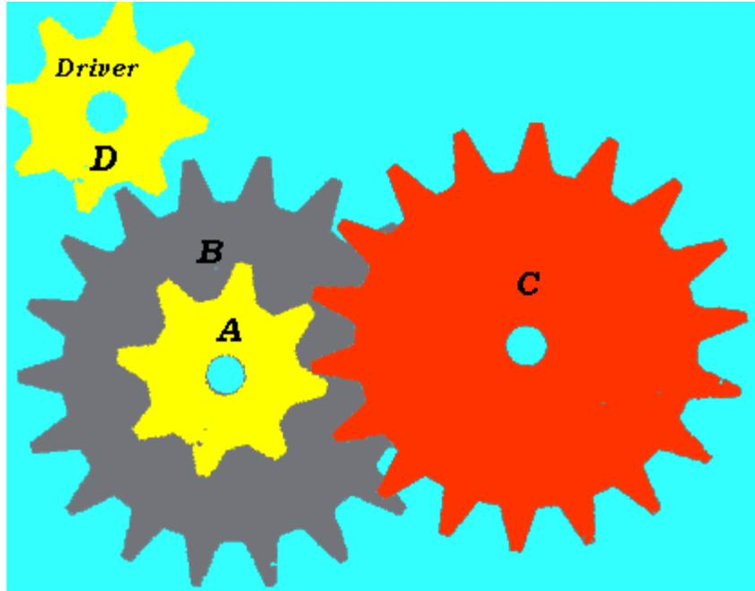
Find Gear Ratio of gear A to gear D
