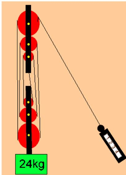
What is the reading on the spring balance attached to the rope where the effort is applied?
