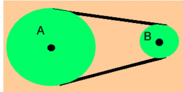
By connecting a large driving pulley to a smaller driven pulley we can increase the number of rotations, change the direction of rotation and reduce the force that is exerted by the driven pulley.
