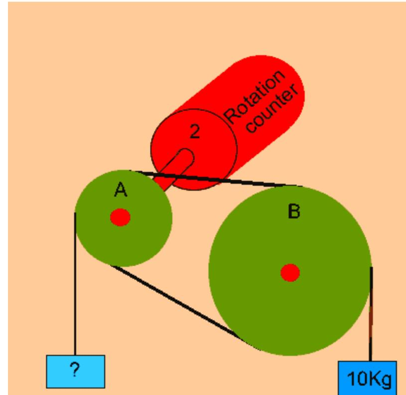
Pulley "A" is connected to the shaft of a motor. The motor can generate enough force to just lift a 8kg mass off the ground when the mass is tied around the shaft of the motor.
