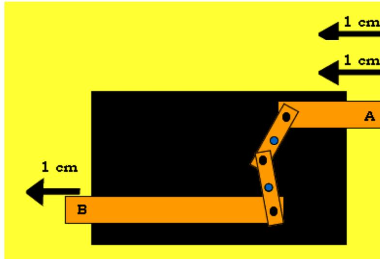
Design a set of levers housed in the black box that will carry out the following functions When lever "A" is pushed in 1 cms Lever "B" moves in 1cm in the same direction.
