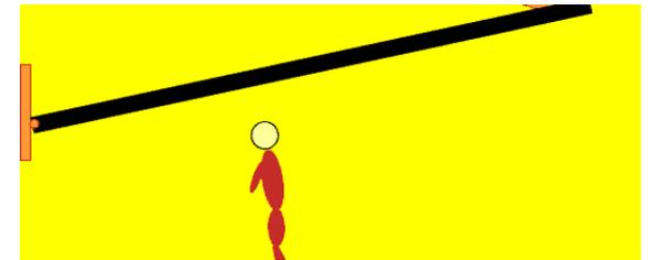
The most simplest of machines is the common lever. A simple log can act to magnify forces and shift objects heavier than the person holding the log. All levers have a **fulcrum** (turning point), **effort** (the force provided to do the work) and the **load** (the force we are pushing against). There are three classes of levers, **first order**, **second order** and **third order**. They differ in the position of the fulcrum, load and effort.
