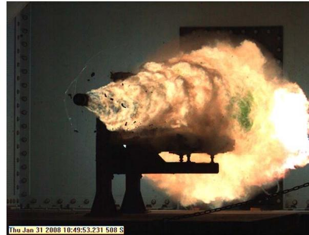
A **railgun** is an [electrically powered](#) electromagnetic projectile launcher based on similar principles to the [homopolar motor](#). A railgun comprises a pair of parallel conducting rails, along which a sliding armature is accelerated by the electromagnetic effects of a current that flows down one rail, into the armature and then back along the other rail
