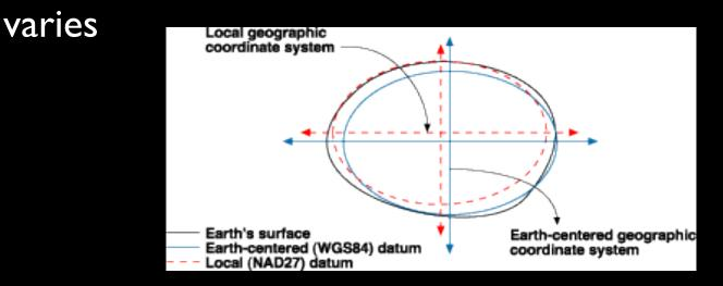
Datums are mathematical models of the shape of the earth created to provide control over the survey measurement framework
