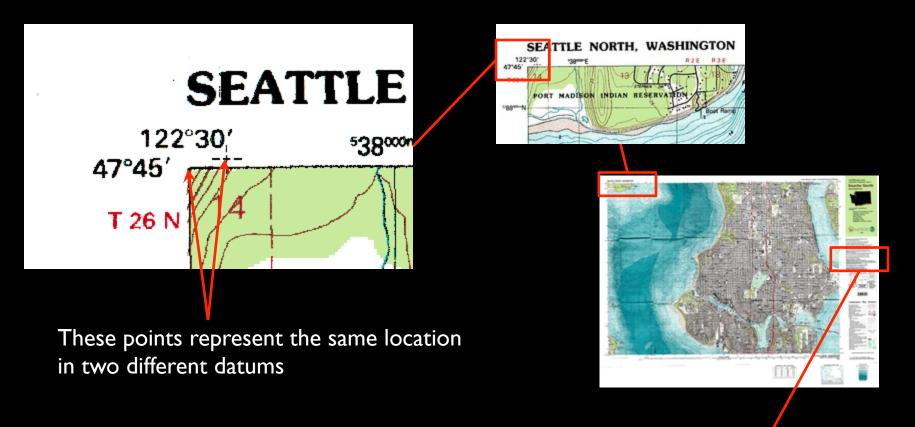
Projection and 1000-meter grid, zone 10, Universal Transverse Mercator 10,000-foot grid ticks based on Washington coordinate system, north zone
