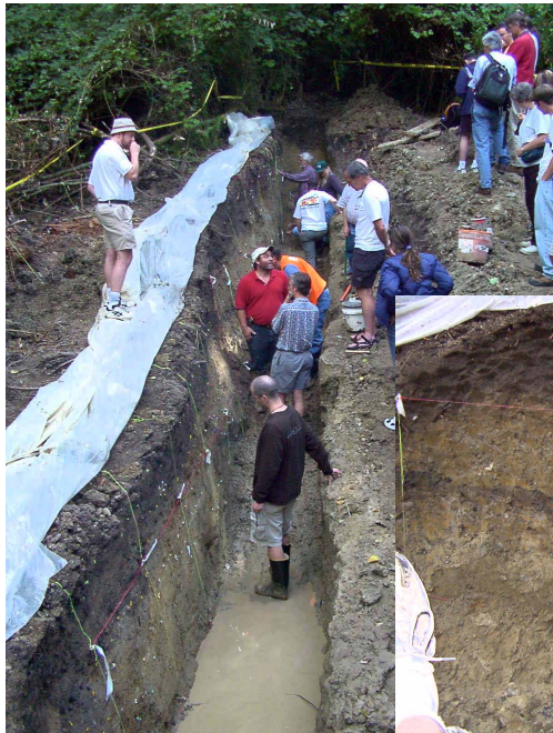
Seattle (reverse) Fault Trench near I90 and Newport Way 1000 year old displacement
