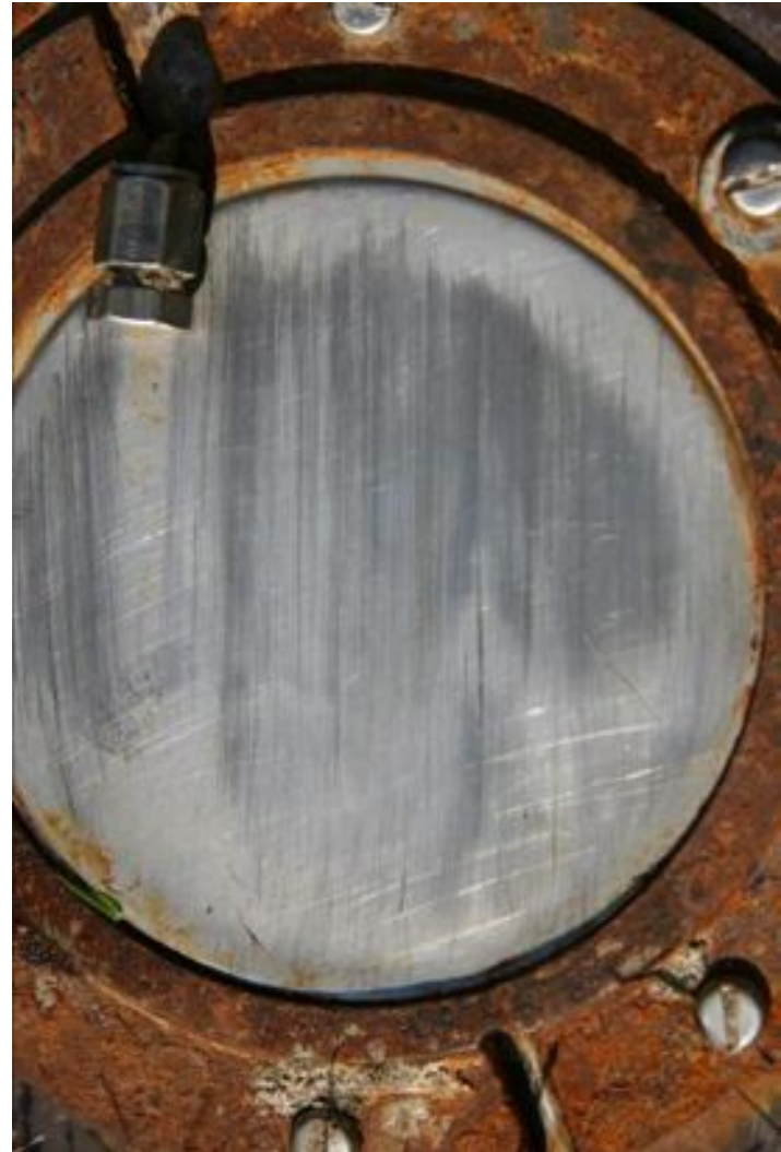
Pressure sensors under 10-20m of ice at Grinnell Glacier: before and after (note abrasion shadows)
