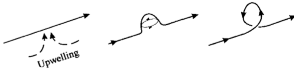
Fig. 8.8. Production of a poloidal magnetic field. A region of fluid upwelling, illustrated by dotted lines on the left, interacts with a toroidal magnetic field (solid line). Because of the Coriolis effect (northern hemisphere) the fluid exhibits helicity, rotating as it moves upward (thin lines, center). The magnetic field line is carried with the conducting liquid and is twisted to produce a poloidal loop as on the right. After Parker (1955a.)
