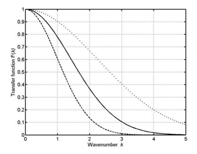
Figure 1. Transfer function F(k) for analytical diffusion equation, as a function of wavenumber k, for time steps  $\Delta t=0.1$  (dotted),  $\Delta t=0.25$  (solid), and  $\Delta t=0.5$  (dashed). Diffusion parameter is  $\Gamma = 1$ .
