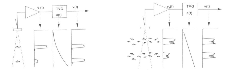
where  $v_1(t)$  = uncompensated voltage, a(t) = receiver gain, v(t) = compensated voltage
