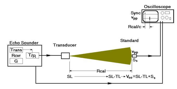
The oscilloscope vpp (volts) is converted to Vso (dBv):
