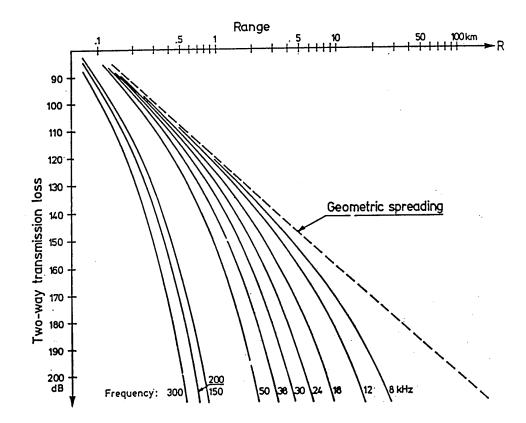
TWO WAY TRANSMISSION LOSS VS. FREQUENCY.
