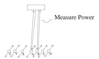
monostatic transducer or transceiver: transmits and receives from same source
