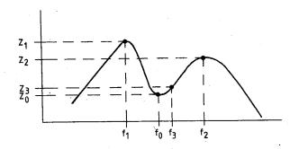
Figure 10c. Typical impedance characteristic.
