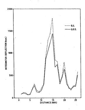
Figure 15. Illustration of echoabundance measures displayed for each mile sailed along a 26 mile obtained course, during the intercalibration "Bjarni of Saemundsson" "G Sars", and October 1982.
