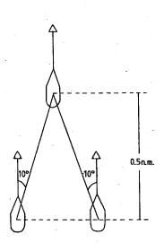
Figure 14. Sailing formation during an intercalibration of three vessels.
