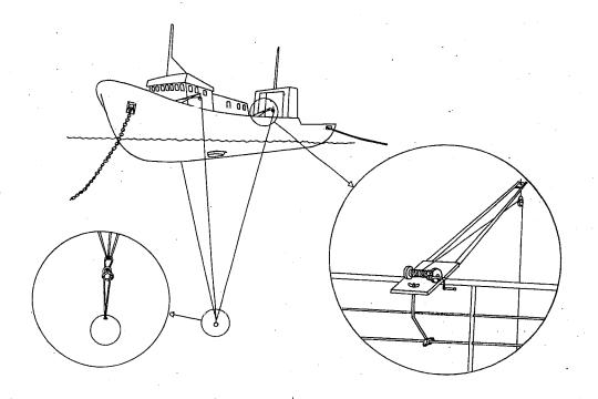
Figure 1. Rigging of a research vessel for stationary-sphere calibration.
