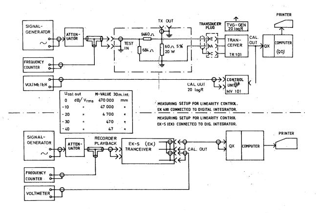
Figure 13. Equipment set up for checking the echo-integrator linearity (ref 3.4.4.3).
