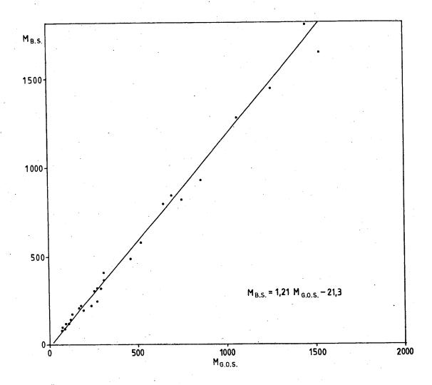
Figure 16. Scatter diagram with regression line of echo abundance measures of "Bjarni Saemundsson" and "G O Sars" during intercalibration.
