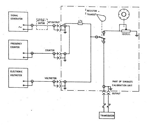
Figure 11a. Instrument configuation for impedance measurement.
