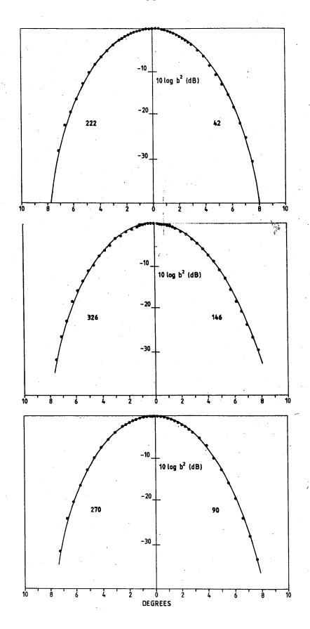
Figure 6. Measured two-way directivity patterns of the 38 kHz hull-mounted transducer on "Bjarni Saemundsson".
