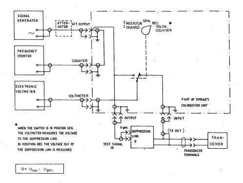
Figure 12a. Equipment set up for measuring the attenuator (ref 3.4.3.2).
