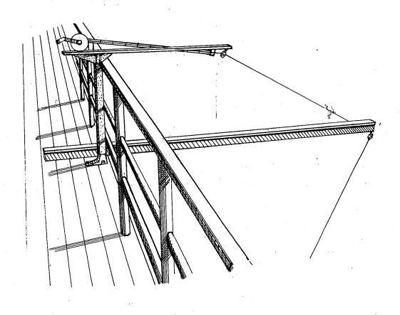
Figure 5. Equipment for transducer beam pattern measurement. The meter rod is used for precise length control of one of the lines suspending the sphere.
