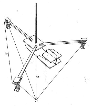
Figure 2. Rig and target suspension for towed-body calibration: moving sphere method.
