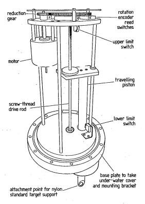
Figure 3. Mechanism for adjusting the length of twine supporting the standard target. Three such adjusters are shown at the arm ends in Figure 2.
