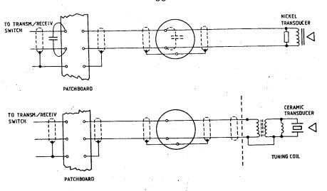
Figure 10a. Principal circuit diagram for nickel and ceramic transducers (ref 3.4.2).
