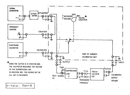
Figure 12b. Equipment set up for measuring the amplification (ref 3.4.3.3).
