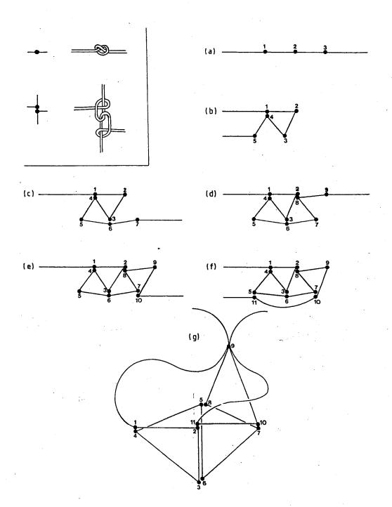
Figure 4. Construction of a monofilament container for standard target spheres. The numbers show the order of tying knots. Successive knots are one quarter of the sphere circumference apart.
