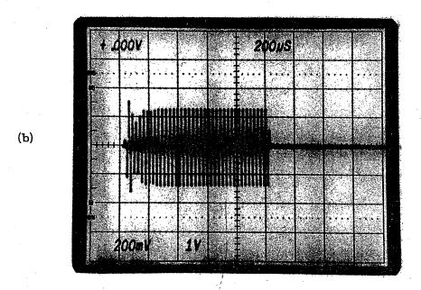
Figure 9. Oscillographs of a 1 ms transmitter pulse measured (a) with a voltage probe; 100 x amplification; scales: 500 V/cm vertical, 0.2 ms/cm horizontal; and (b) with a current probe, conversion factor 10 mA/mV; scales: 10 A/cm vertical, 0.2 ms/cm horizontal.
