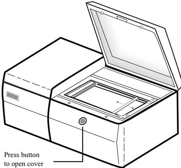
**Figure 3-4. Front view of FMBIO scanning unit**
