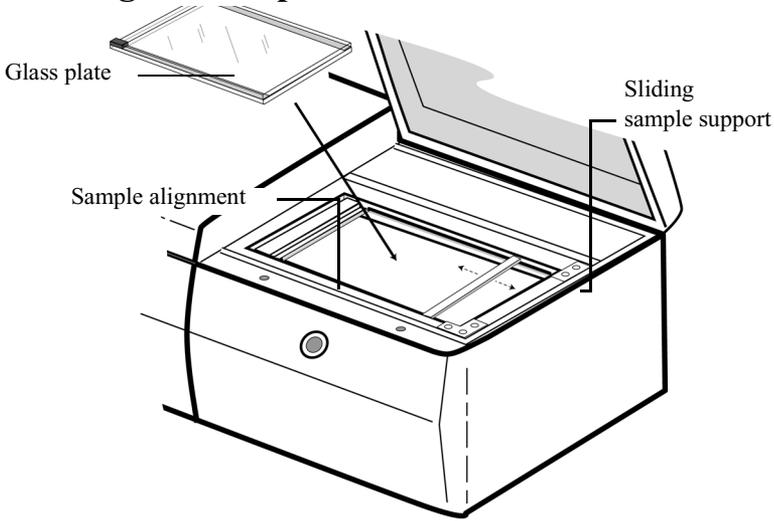
**Figure 3-5. Loading the glass plates on to the scanner bed**
