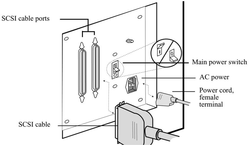
**Figure 3-2. Rear view of FMBIO scanning unit**
