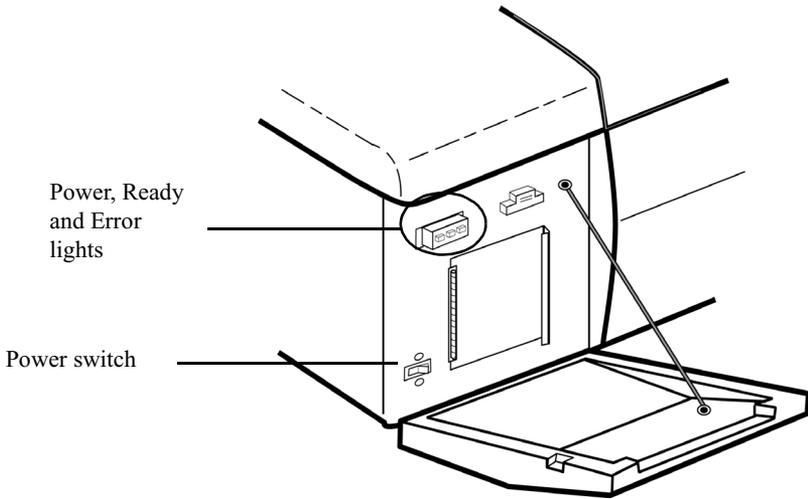
Figure 3-1. Inside front panel with Power switch
