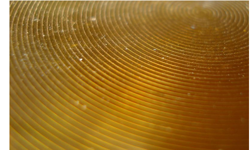
Close-up view of a flat Fresnel lens shows concentric circles on the surface
