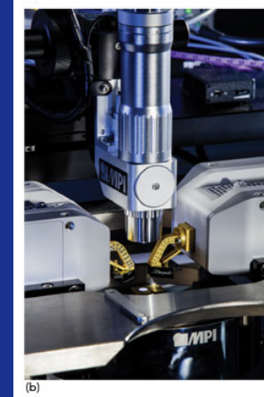
(a) R&S ZNA vector network analyzer. (b) R&S ZNA with MPI TS150-THZ integrated probe system for 330 GHz measurements
