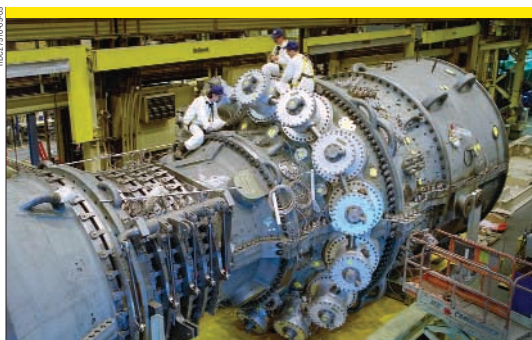
A 9H gas turbine is readied for testing.
