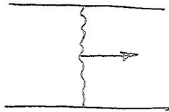
Speed with which a vanishingly small disturbance moves to right.
