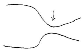
The throttle has negligible KE on either ends so  $T_{in} = T_{out} = T_0$
