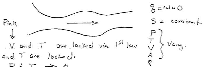
Note that  $q = w = 0$  means  $V$  and  $T$  are locked via 1<sup>st</sup> law
