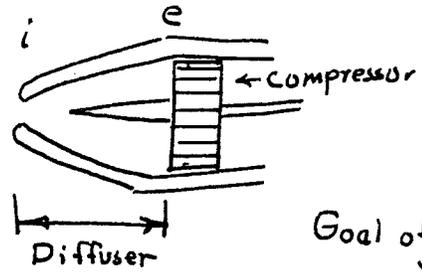
Goal of the diffuser is to recover the incoming velocity to preheat & pressurize gas.
