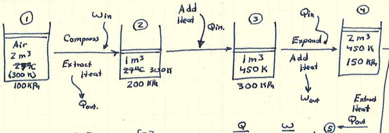
$1-2 \quad P_2 = P_1 \left[ \frac{V_1}{V_2} \right] = 100 \text{ kPa} \left[ \frac{2}{1} \right] = 200 \text{ kPa} \quad \frac{Q}{-138.6} \quad \frac{W}{-138.6}$
