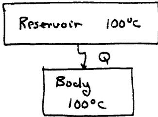
Reversible: No  $\Delta T$ , no work needed to reverse heat flow.
