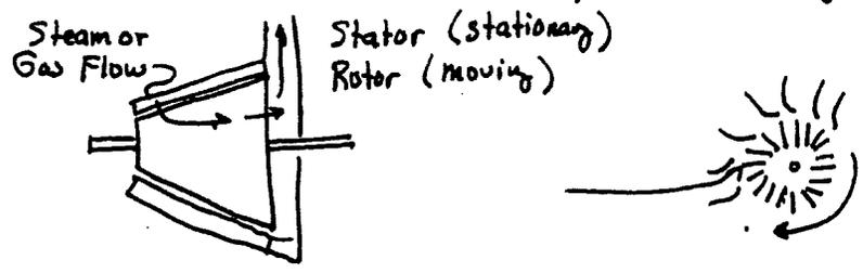
• Inside vanes are straight because curved vanes have problems with centrifugal force.
