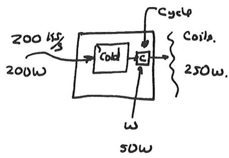
$$\beta = \frac{Q_{in}}{W_{net}} \Rightarrow W_{net} = \frac{Q_{in}}{\beta} = \frac{200 \text{ kJ/s}}{4} = 50 \text{ W.}$$
