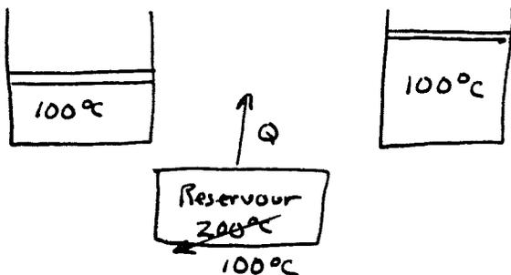
Cannot reverse because  $Q$  won't go from  $100^\circ\text{C} \rightarrow 200^\circ\text{C}$
