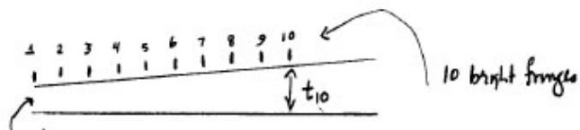
$$\begin{aligned} 2nt_1 &= m\lambda \\ 2nt_0 &= (m+9)\lambda \end{aligned} \quad \left. \begin{array}{l} \Rightarrow 2n\Delta t = 9\lambda \\ \Delta t = \frac{9\lambda}{2n} = \frac{9 \cdot 630}{2(1.5)} = 1890 \text{ nm} \\ = 1.89 \mu\text{m} \end{array} \right.$$
