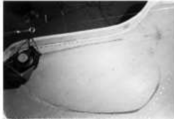
Fig. 17. First (lowest) soundboard mode at 49 Hz.
