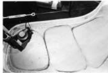
Fig. 19. Third mode at 89 Hz.
