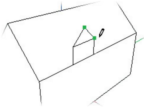
Now that we have the front part as a framework, let's draw in the ridge line of the dormer. SketchUp will help you find the point where the ridge will hit the plane of the roof with the 'On Face' ToolTip and a blue inference point. Make sure you are aligned parallel to the appropriate axis as well.
