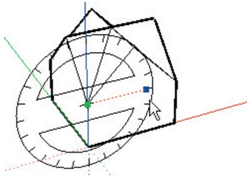
At this point a construction line appears through the center of the Protractor. Use the cursor to snap the indicator line to the roof edge. The size of the angle is displayed in the Value Control Box. If you see a value of 45 degrees, you have used the Protractor tool correctly. Click the mouse to set a construction line at this angle if you need one, otherwise press Escape to cancel the operation.
