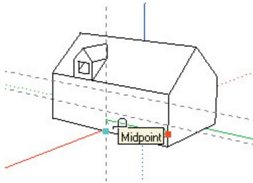
Activate the Rectangle Tool. Start from the intersections of your construction lines, then move your cursor to the other parallel construction line. Watch the VCB to make the window 3' tall and 4' wide, or type in ( 4',3' ) and press Enter.
