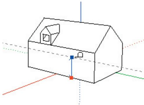
Now type 6'8" (this will appear in the Value Control Box) and press Enter. Your Construction Line will snap to exactly 6'8" above the bottom edge.
