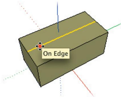
Go ahead and click on the line and move the mouse upwards. To make certain you are moving the line straight up, watch for the blue inference line as well as the 'On Axis' selection tip. This will form the peak of a simple gable roof.
