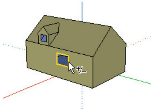
Next, activate the Move Tool, and click on one of the window's corners. Using a linear inference, drag the window into alignment with the dormer above. Click the mouse button again to complete the move operation.
