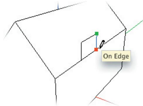
Next, create a vertical inference line from the midpoint of the top edge of the rectangle. To do this, move your mouse over the midpoint snap on the edge without clicking, then move the cursor up. SketchUp will show you it has inferred the proper alignment with an inference point and the 'From Point' ToolTip.
