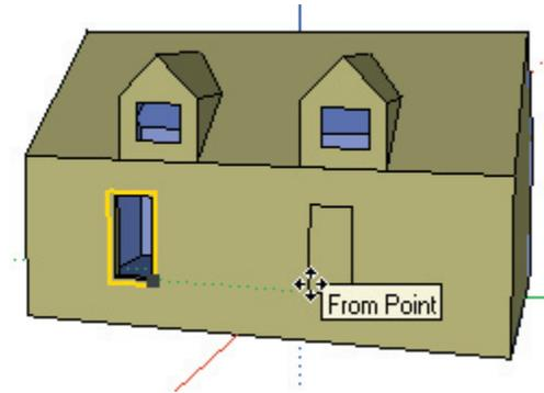
Notice the window cuts a hole in the wall for you, just like the dormer.
