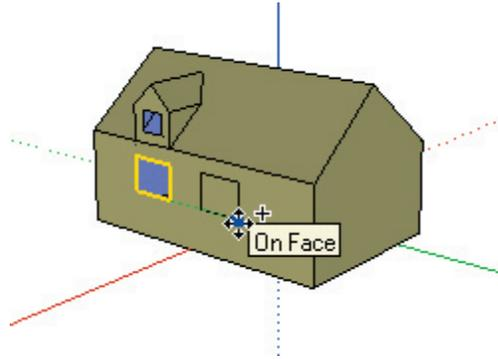
Release the Ctrl key, and type '7' followed by Enter. Notice that when you have copied the window lines, the hole (or absence of a face) is copied as well.
