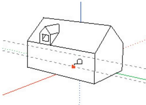
These two construction lines will help us place the top and bottom edges of the windows accurately.
