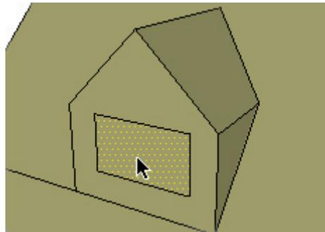
When it is highlighted, delete it by pressing the Delete key. You should see a hole in the front face of the dormer. Now select the portion of the roof you see inside the dormer and delete it too.
