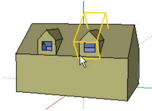
Notice that the roof has been properly trimmed by the component- Just as it was in the original dormer.
