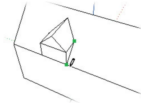
To complete your simple dormer, activate the Erase Tool and erase the unnecessary line in the front face of the dormer.
