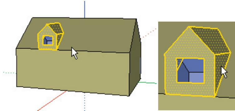
Notice that the roof plane has been cut away within the dormer to create a "hole" in the roof. The edges which touch the roof plane form the border of this hole. This behavior will become part of the Component definition.
