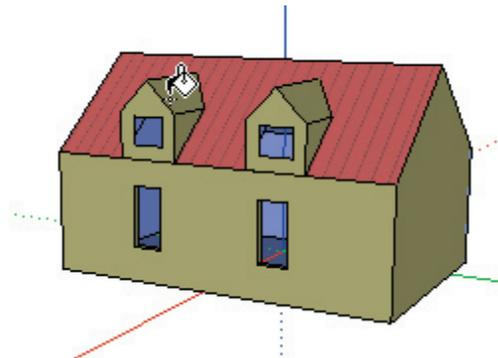
Now right or Control-click on a dormer and select 'Edit Component'. Once inside the Component context, select the StandingSeam material and paint it onto the roof surfaces of the dormer.
