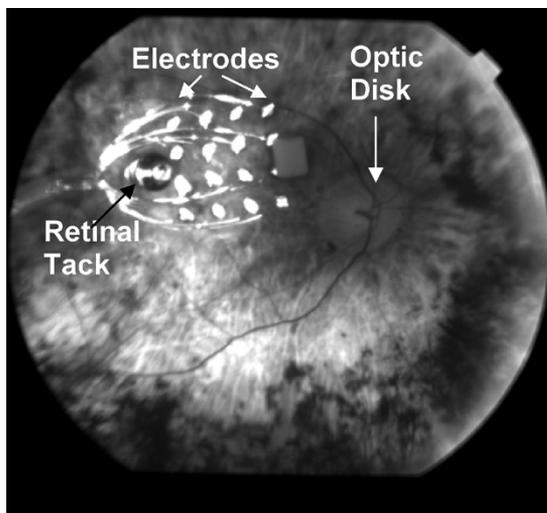
Fig. 1. Fundus photograph of an intraocular stimulating array viewed through a dilated pupil. Sixteen platinum electrodes are held on the retina with a single retinal tack.
